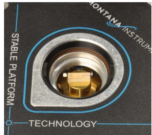
Figure 2. Vertical viewing, high NA (microscope type application) Sample is mounted on top and positioned just inside warm window.
